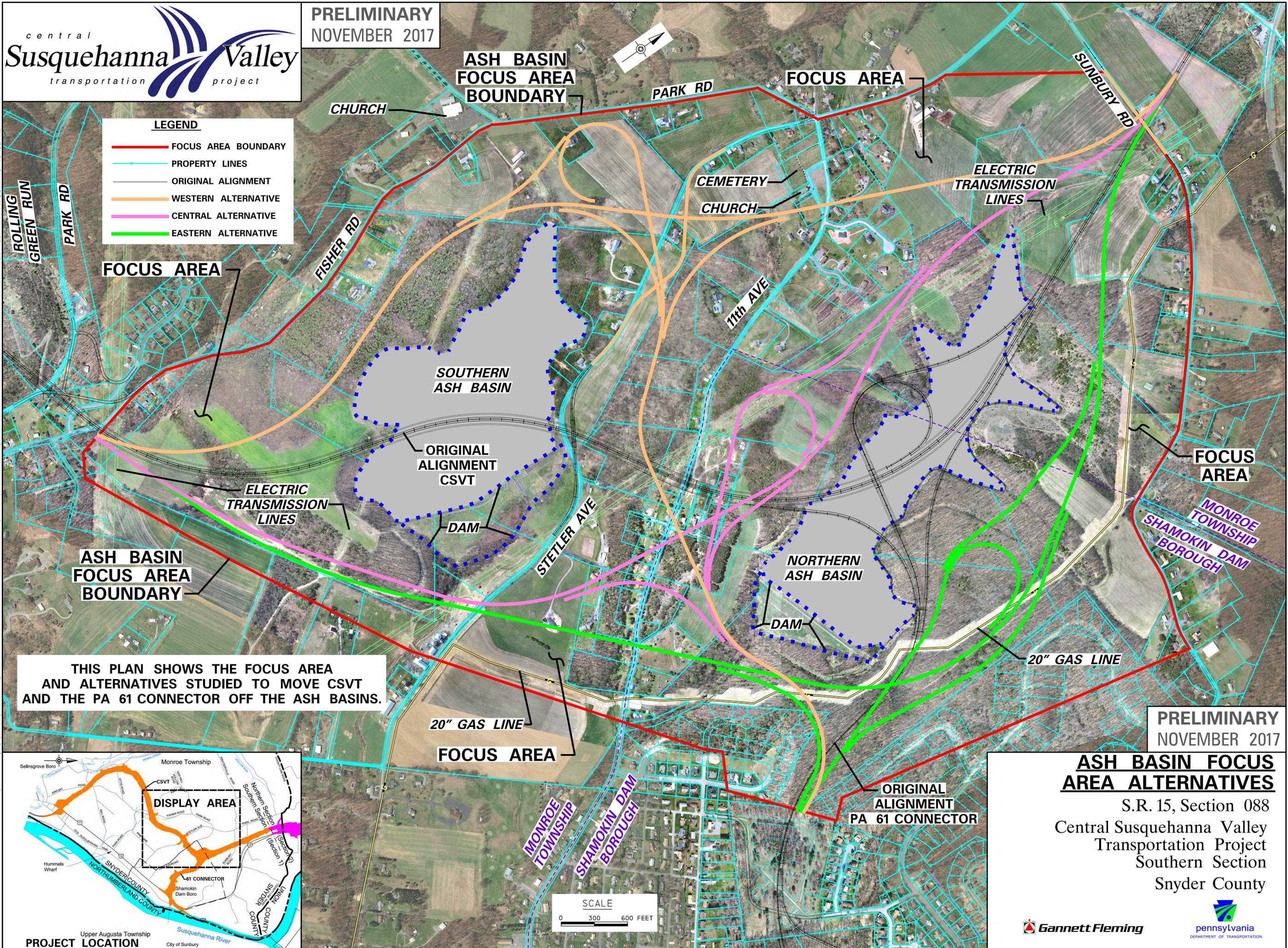
THIS PLAN SHOWS THE FOCUS AREA AND ALTERNATIVES STUDIED TO MOVE CSVT AND THE PA 61 CONNECTOR OFF THE ASH BASINS.
